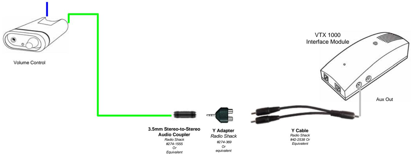
1. Connect the stereo coupler to the cable with the green mini-plug attached to the MicroWorks II volume control
