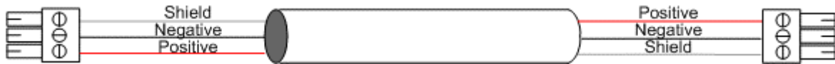
Figure 29. Building a cable for the balanced to balanced connections on the Vortex and VSX 8000.
