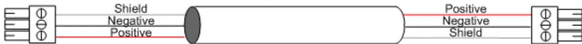
Figure 30. Building a cable for the balanced to balanced connections on the Vortex and VSX 8000.
