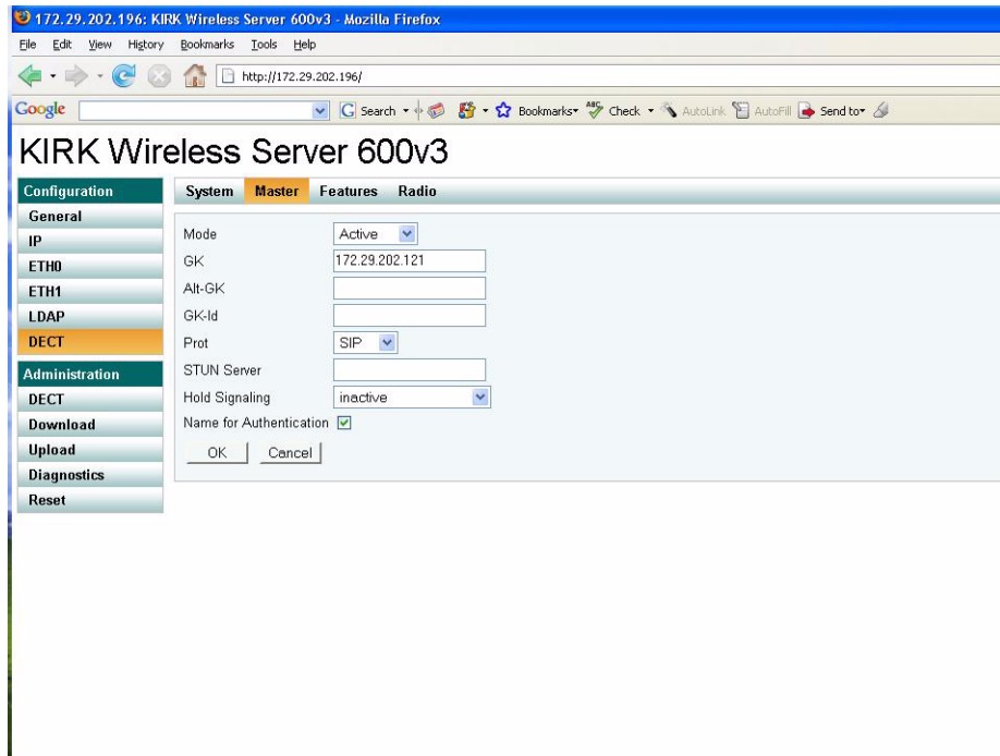
Figure 2-1 Adm. Page: Configuration/DECT/Master page - SIP Protocol on Samsung OS2700 SW 4.11
