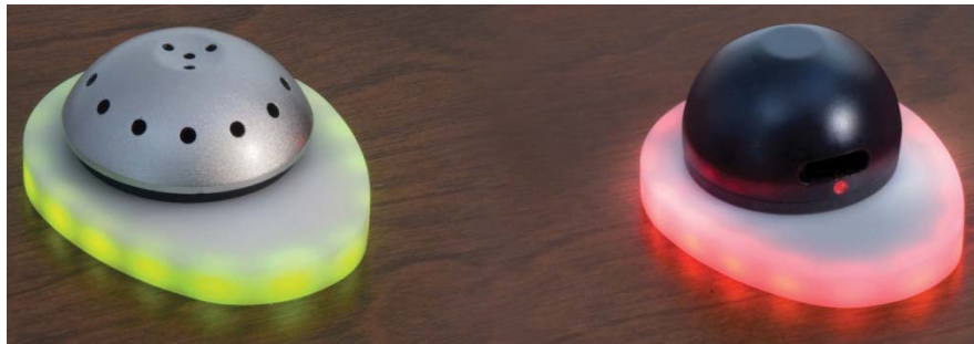
Figure 1. Two Clockaudio Litetouch Halo ring and touch pads with through-table microphones with green (left) and red (right) LEDs illuminated [1].
