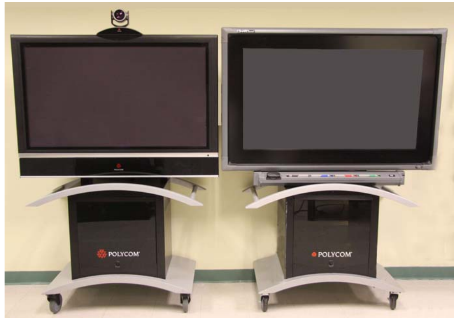
Figure 1-1 Instructor FS HDX Dual Display on the Media Cart with People Display (on Left) and Content Display (on Right)
