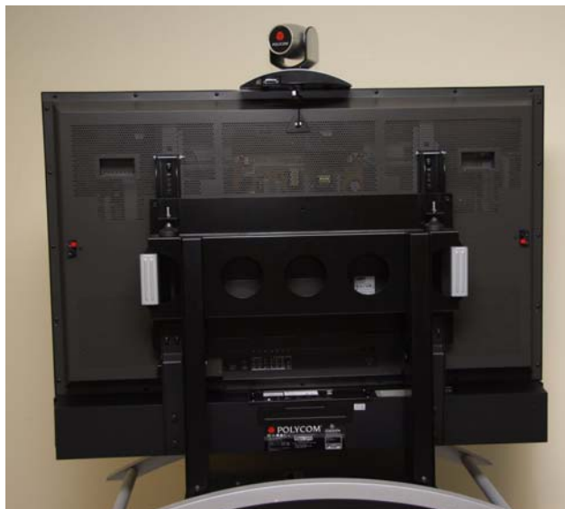
Figure 2-6 Attaching the Camera to the People Display
