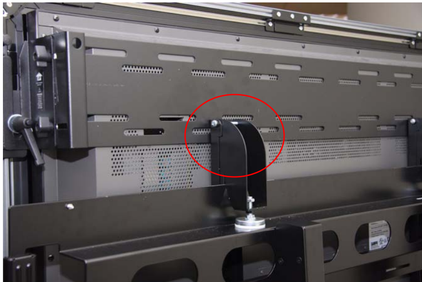
Figure 2-7 Attaching the SMART Board Brackets and the Monitor Brackets
