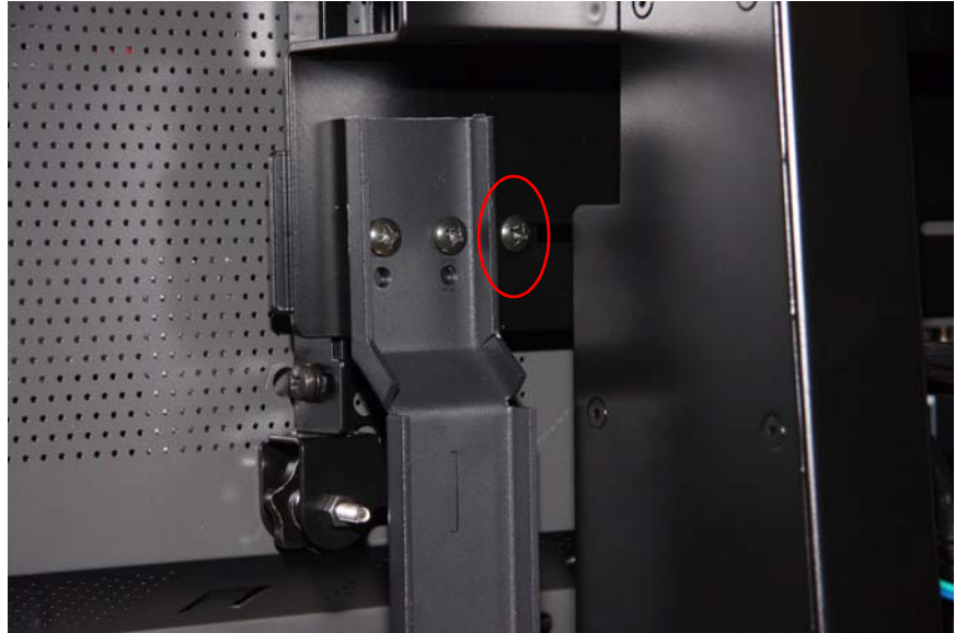
Figure 2-3 Attaching Screws to Stabilize the People Display
