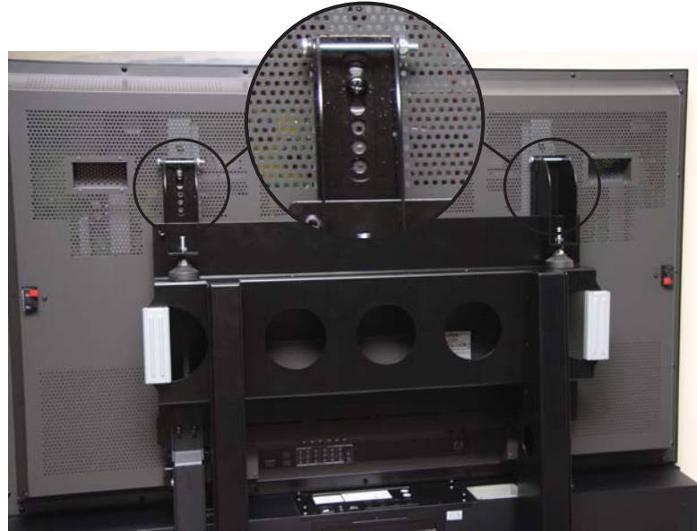
Figure 2-1 Attaching the Monitor Brackets to the People Display
