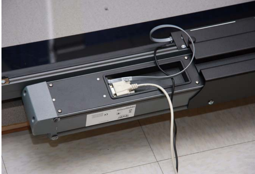
Figure 2-11 Attaching the Cables to the SMART Board Overlay
