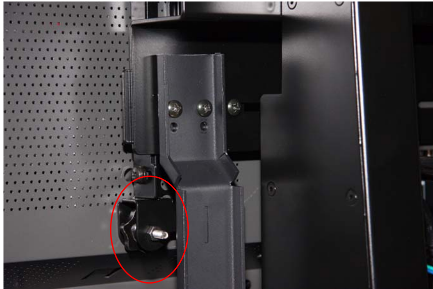
Figure 2-8 Adjusting the Display Tilt Angle
