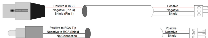
Figure 6. Balanced microphone input to balanced input on Vortex (top) and unbalanced to balanced recommended wiring (bottom).
